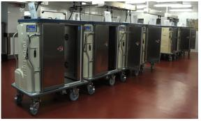
Recently installed energy efficient rethermalisation food carts (above) provide energy savings of 157,089 kWh per year; a 71.73 kW energy demand reduction when compared to the old equipment.
