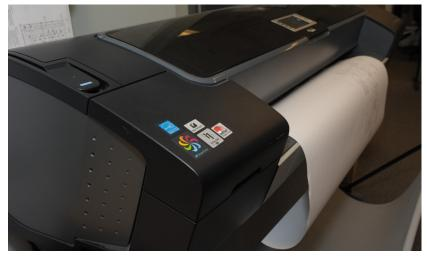
In addition to making prints that resist fading for over 200 years, this ENERGY STAR qualified Hewlett-Packard Designjet plotter, used by the TOH Engineering & Operations Group, produces less heat, consumes only 200 watts of energy when active; 27 watts in powersave mode, and 43 watts on standby. This is one of two highly energy-efficient plotters in use at TOH.
